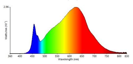
Testing was performed in accordance with LM-79-08.
